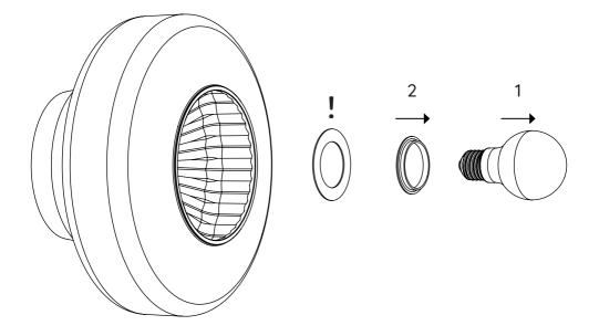
1 Loosen the light bulb and remove it.
