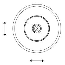
Slightly loosen the socket ring and move the glass to the desired location. While holding the glass in position, tighten the socket ring. Keep in mind that all lamps are handmade which means that it might not be possible to adjust it perfectly centered.
