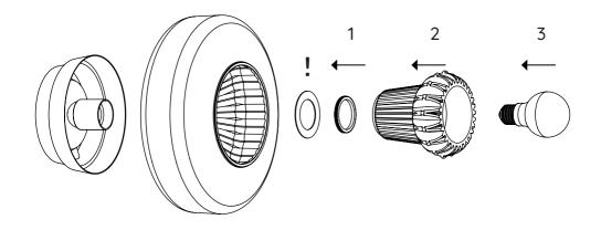
! Make sure that the rubber spacer is placed between the lamp glass and the socket ring.
