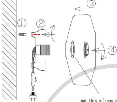
put this silicon sheet here which can avoid touch between glass and sockt cup
